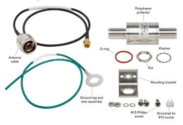
Campbell Scientific surge protector kits protect RF equipment by equalizing the potential difference between the centre pin of the coax cable and its shield. The kits include a capacitive-coupled gas tube protector with multi-strike capability. If properly grounded, the capacitor will block low frequency surge currents induced onto the centre-pin from the antenna side until the gas tube reaches a high enough voltage to shunt the surge to ground.
